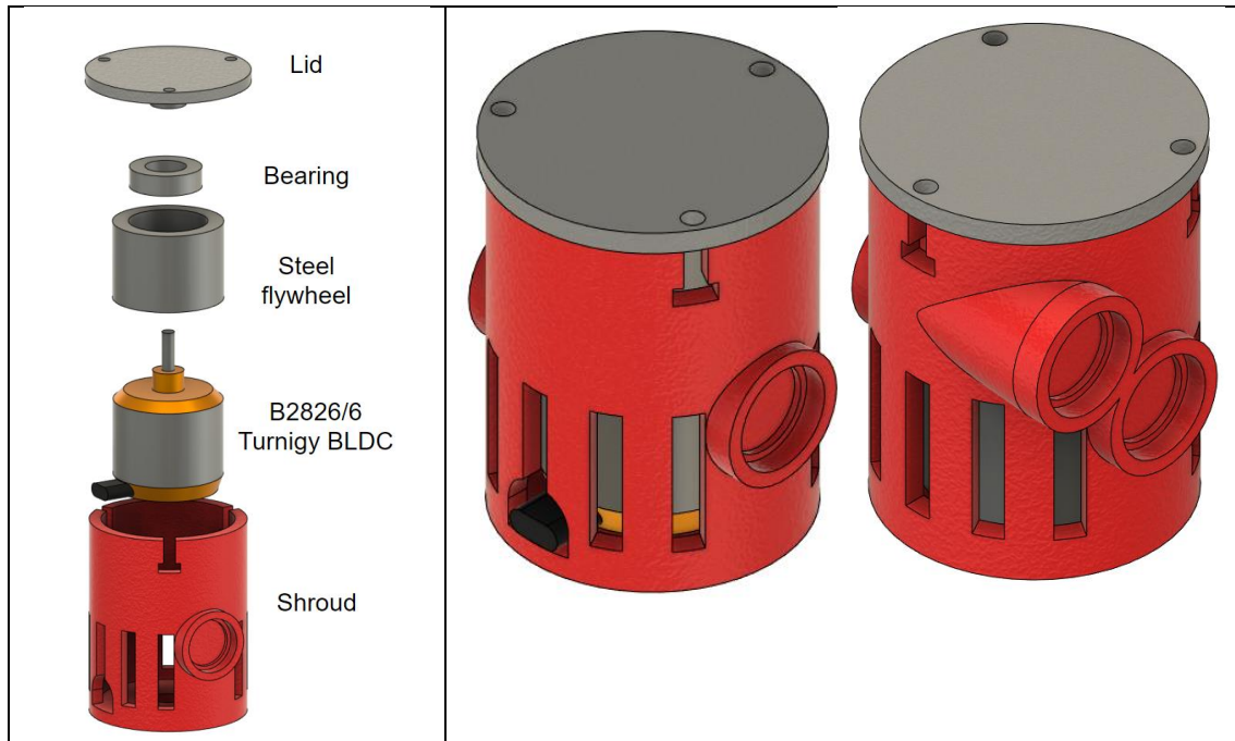
Figure 17: exploded diagram of flywheel assembly (left), and shroud design (right).
