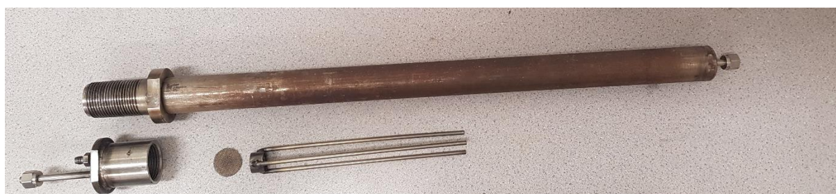
Figure 3.4: Stainless steel reactor tube ( \varnothing 40 mm, L = 500 mm) with nitrogen port at the bottom (right). On the right, screw-on lid with gas outlet port and thermocouple port. Also, 150 mm long sample stand (tripod) with mesh tray (No. 35 sieve size).
