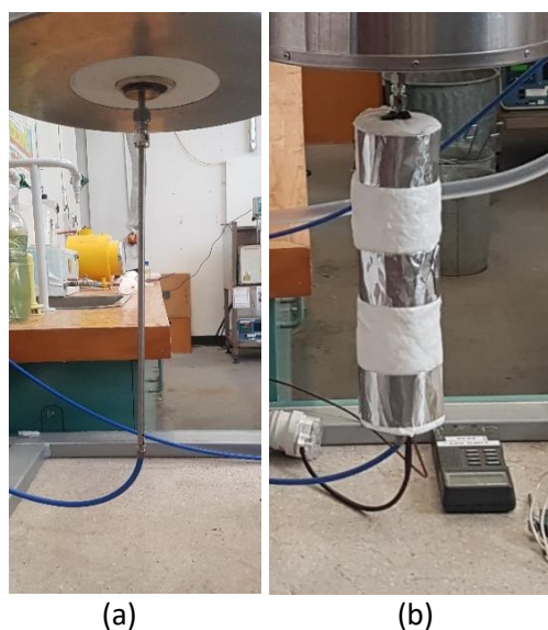
Figure 3.3: Nitrogen feed into the bottom of the reactor. Set up for (a) initial design without preheating installed, and (b) final design with preheating (to 200°C) installed and insulated.
