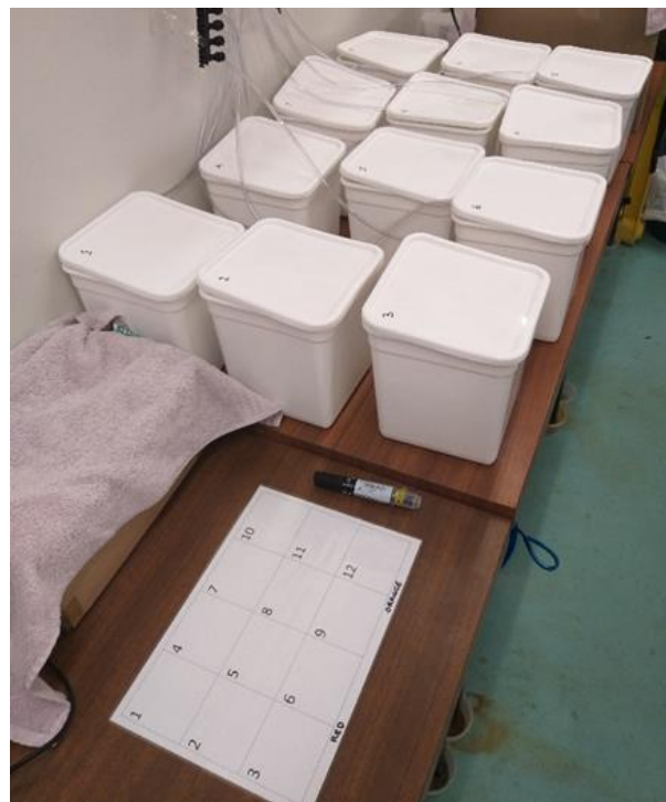
A1 Figure 2. Aerated and temperature-controlled recovery tubs in which fish regained equilibrium post- CT_{max}
