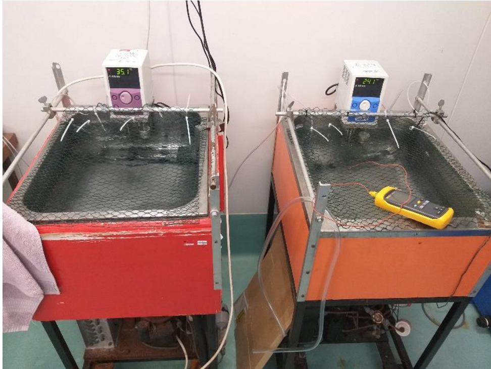
A1 Figure 1. Custom water baths used for controlled temperature ramping during CT_{max} trials.
