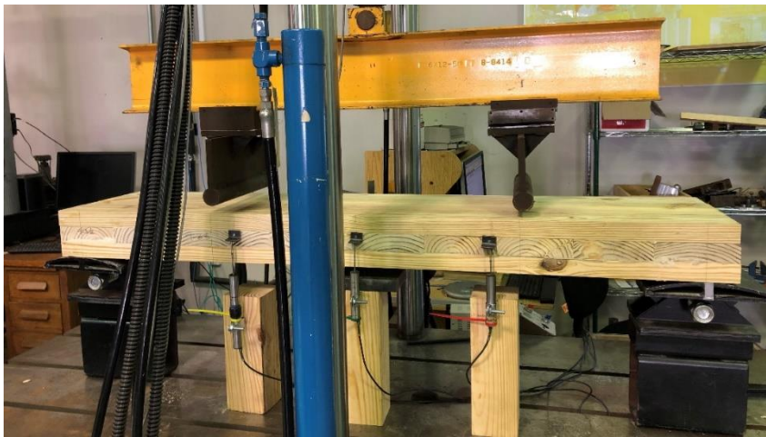
186 187 Fig. 3. Four-point CLT bending test setup
