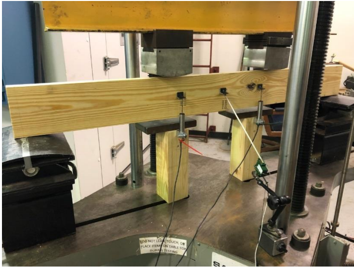
161 Fig. 2. Non-destructive edge-wise four-point bending test set-up
