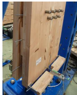
Figure 7: CLT5 (panel splitting)
