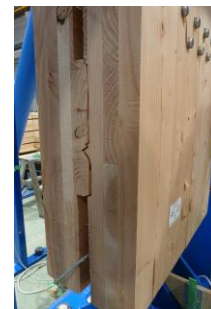
Figure 8: CLT7 (panel splitting)
