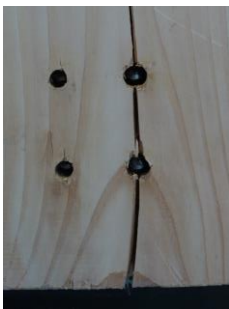
Figure 6: CLT3 (row shear)
