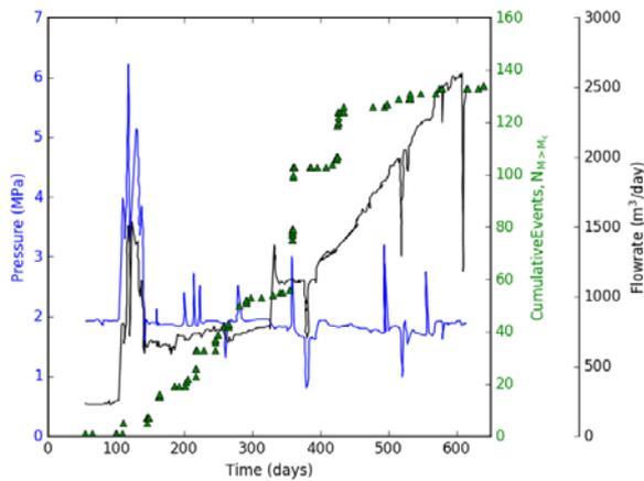
**Figure 4: Wellhead pressure (MPa), Injection Rate (m<sup>3</sup>/day) and detected seismic events of RRG-9.**
