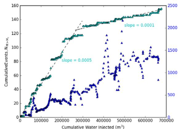
**Figure 7: Modified hall plot (Eq. [2]) of seismicity and cumulative water injected (m<sup>3</sup>) for all seismicity at RRG-9.**
