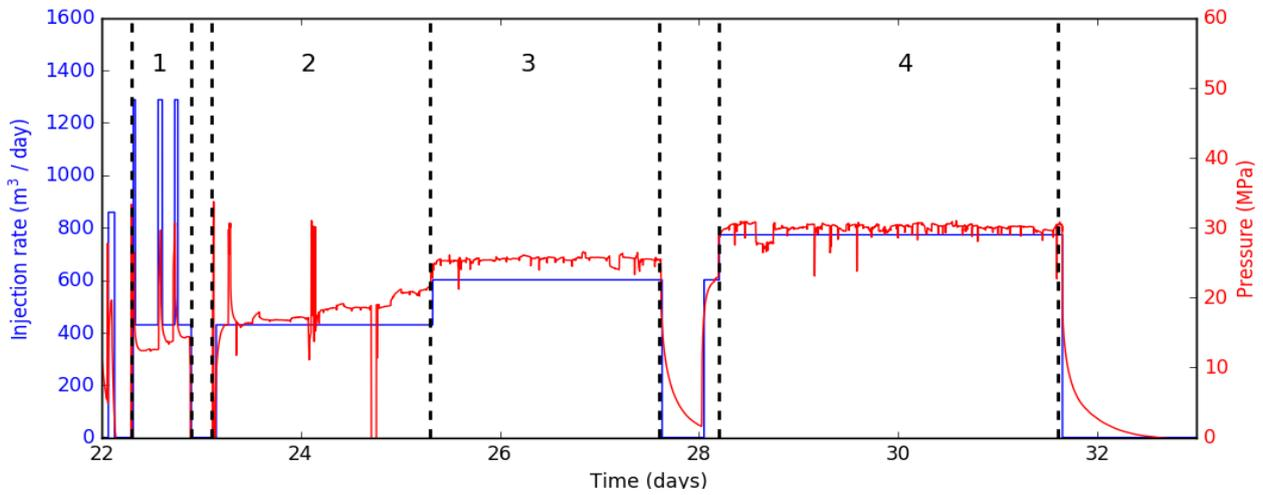
**Figure 1: Wellhead pressure (MPa) and injection rate (m<sup>3</sup>/day) plotted against time for stimulation of the Habanero-1 well, Cooper Basin, South Australia. Time, in this case, is the period in which the step-rate injection was performed in the span of the overall 40-day injection. Dashed lines and numbers indicate four periods of constant flow rate injection and are these are replicated, for reference, in later figures.**
