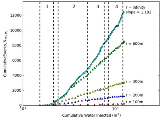
**Figure 3: Modified hall plot (Eq. [2]) applied to Habanero-1 for seismicity within different radial distances,  $r$ , from the wellbore plotted on linear (left) and logarithmic axes (right). Dashed lines delineate the different injection rate steps.**
