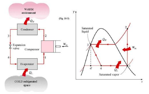
Figure 10: a) Heat pump schematic. b) Vapour compression cycle
