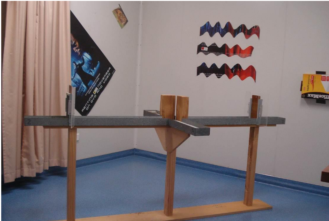
Figure 2.10. Photograph of the elevated cross-maze. The picture shows the two possible starting areas with removable guillotine doors leading down the stem to two reward arms each with a small food tray at the end. Both the stems and arms could be blocked off with use of a large wooden block shown in the picture.
