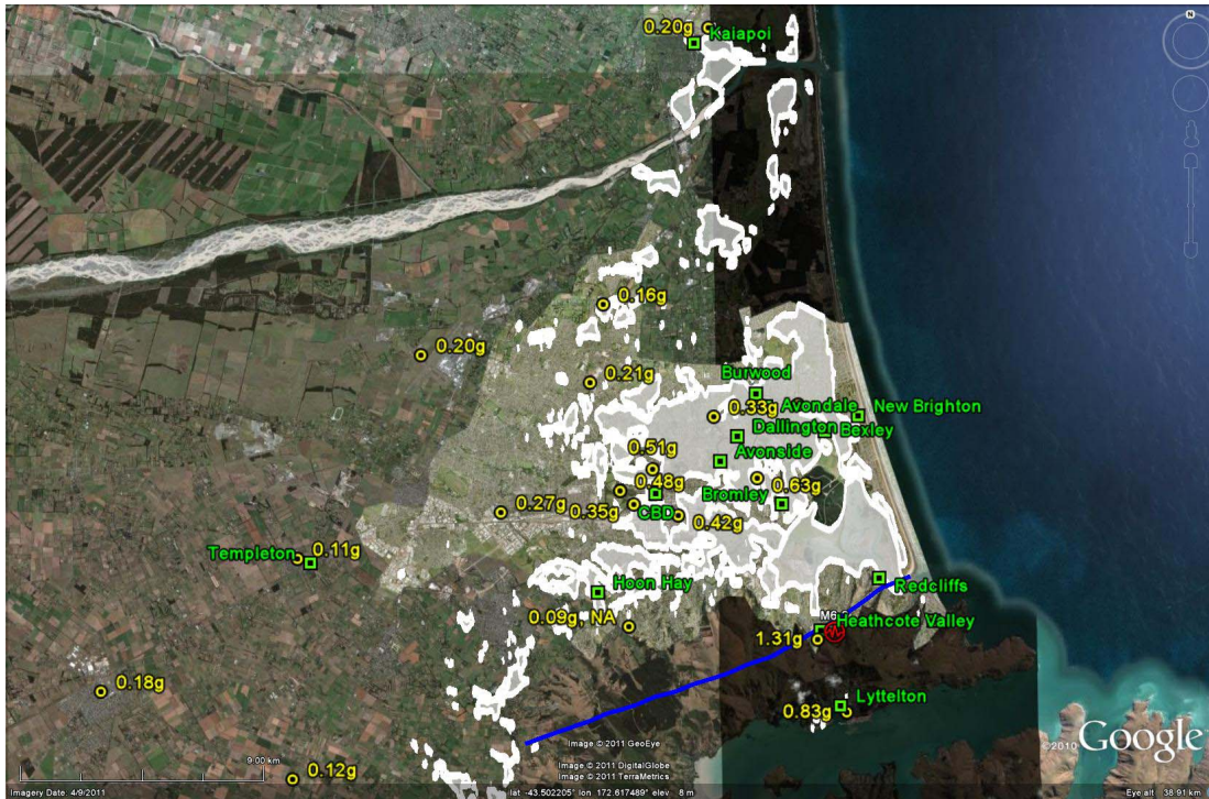
Figure 1. Aerial image of Christchurch showing the ruptured Port Hills fault segment, epicenter, strong ground motion stations and the geometric means of peak horizontal accelerations, and zones that liquefied (white shading).
