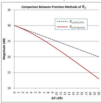
Fig.1 Comparison between  $R_{ij,Proposed}$  and  $R_{ij,EN12354}$  where  $R_{ij} = -10 \log \tau_{ij}$  and  $\Delta R = 10 \log \left(\frac{\tau_{ji}}{\tau_{ij}}\right)$ . The initial value of the calculations was set to  $R_{ij} = R_{ji} = 30 \text{dB}$ .
