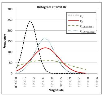
Fig.3 Comparison between the histograms of  $\tau_{ij}$ ,  $\tau_{ji}$ ,  $\tau_{ii,Proposed}$  and  $\tau_{ii,EN12354}$ .
