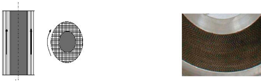
(a) Cross-sections through RPS along and perpendicular to the axis of rotation.
