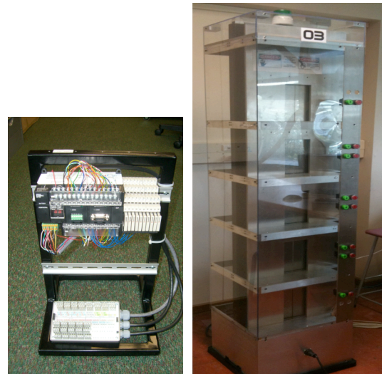
Figure 1. Elevator control project using PLC (left) and tested on the model elevator (right).
