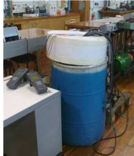
Figure 11. The Dewar used for containing the liquid nitrogen during testing
