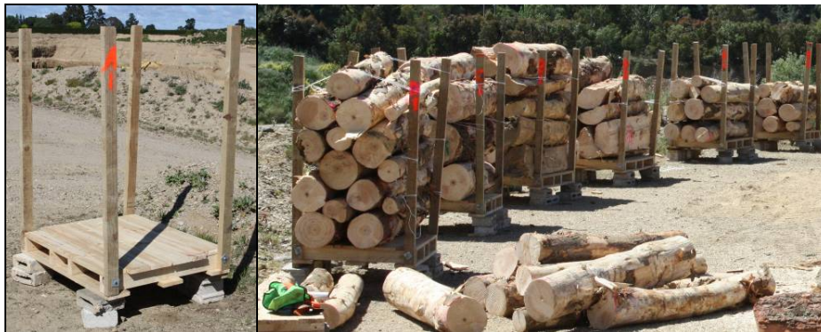
Figures 3a and b: One of the 12 pallets with fitted uprights situated on cinder blocks; and pallets being loaded with logs prior to covering.
