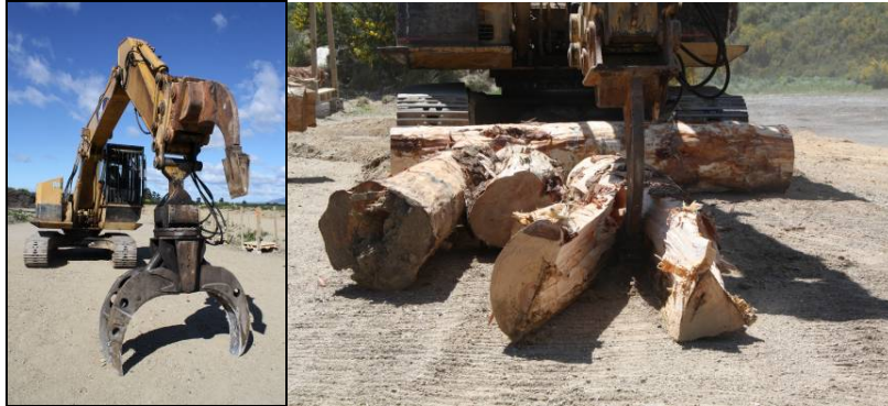
Figures 2a and 2b: The excavator, with attached ripping tine, used for the unloading, handling and splitting of the logs.
