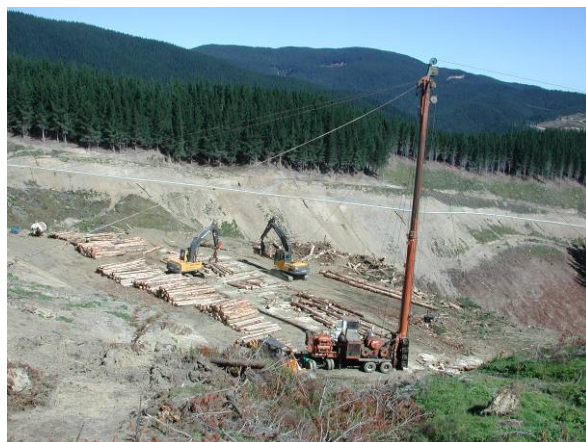
Figure 1: A typical (cable yarder) skid-site that incorporates all the extraction, processing and loading out phases of the operation.
