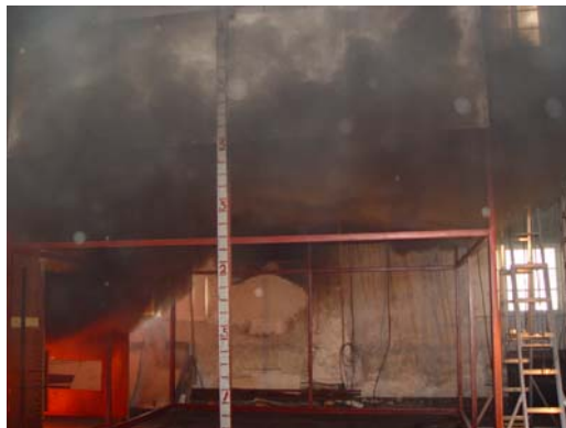
(a)Smoke layer remained stable
