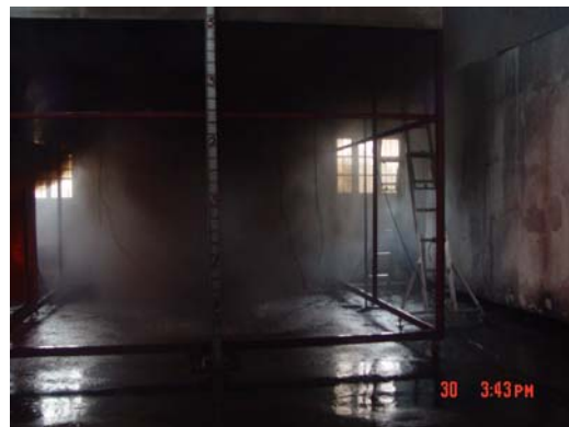
(c) Smoke reaching the floor
