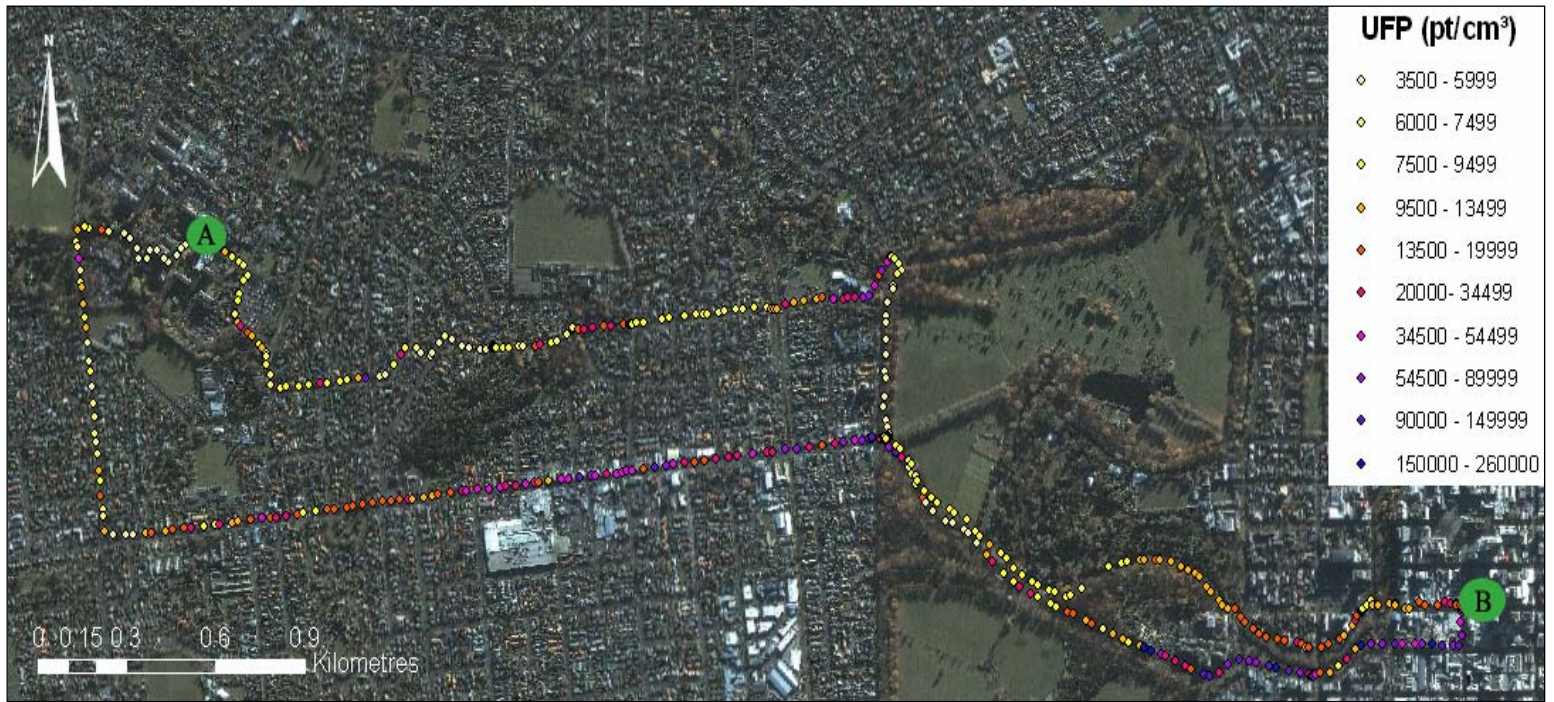
Figure 34 Cyclists' real-time comparative UFP exposure by GPS co-ordinates: Canterbury University to Christchurch city centre, 4:45 – 5:05 pm, 17 March 2009
