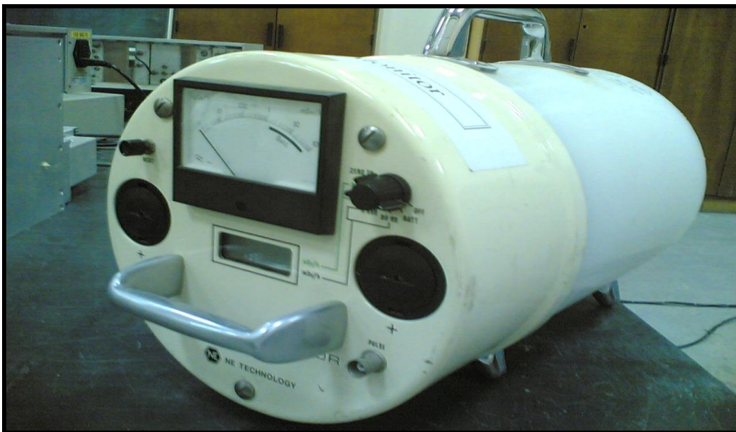
Figure 2.2: Neutron dosimeter detector (NM2B), Serial No. 433[67].
