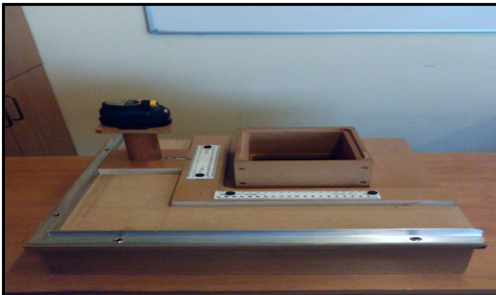
Figure 3.3: Alignment of tumour vessel scale with laser beam pointer.
