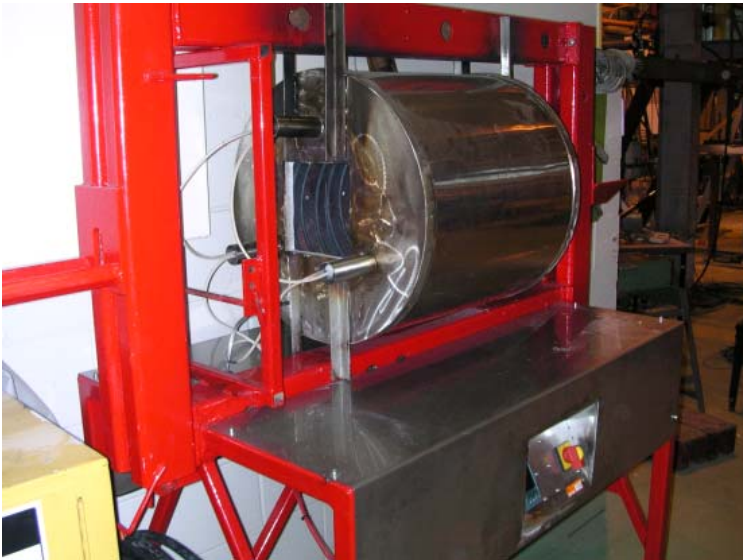
Fig. 2 The test frame and furnace used for the heated tests and fire testing.
