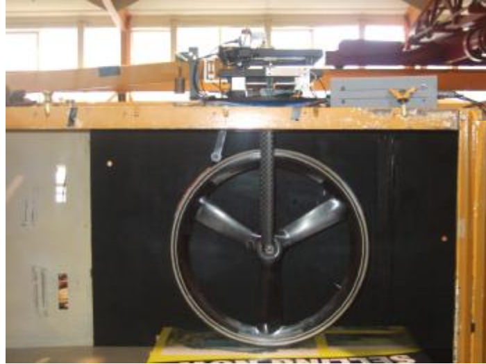
Figure 3.4 Test rig with wheel mounted in wind tunnel
