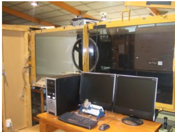
Figure 3.3 PC, test rig, rig motor controller and wheel
