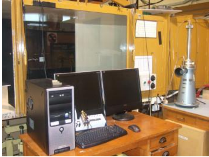
Figure 3.2 PC, data acquisition unit, manometer and wind tunnel speed controller
