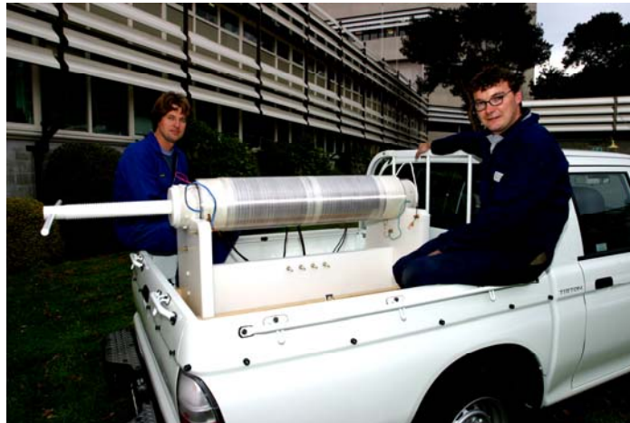
Figure 1 A Light Utility Vehicle Transporting the Dry Type Open Core Resonating HV Transformer
