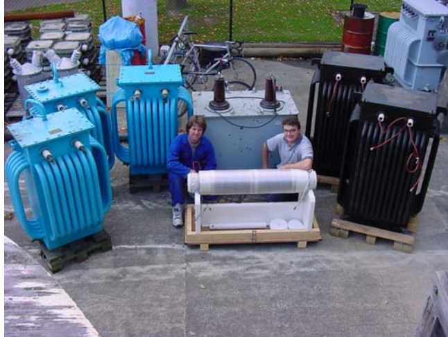
Fig. 2 Manapouri resonant transformer in front of equipment previously used at Tekapo power station.
