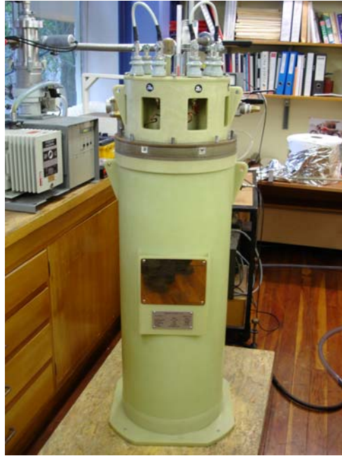
Fig. 3 Partialcore High Temperature Superconducting Transformer
