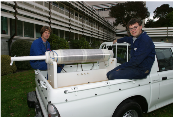
Fig. 1: A light utility vehicle transporting the dry-type open core resonating HV transformer.
