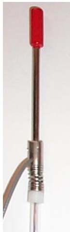
Figure 12: Diode detector mount with spring switch collision detection. An RFA diode (red) is mounted. A post protrudes through the spring into a cup machined into the inside of the diode holder (which has a grey cable exiting on the left).
