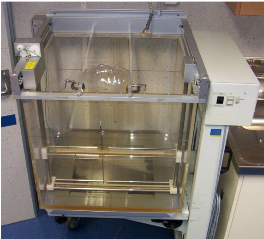
Figure 8: An early configuration of the water tank system, showing a mask in position for scanning and a single Scanditronix diode detector beneath.
