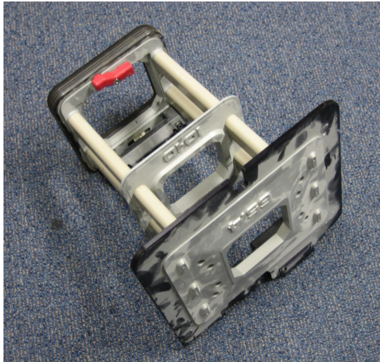
Figure 39: A disused Varian electron applicator. The top scraper is at lower right in this image, and the bottom scraper where an electron cutout or insert would be mounted is towards the upper left. The field size set by this applicator, 10x10cm, is embossed on the middle scraper. This applicator is designed to be mounted 65.4cm (embossed on the top scraper) from the reference origin of the linac head, which is taken from the top surface of the x-ray target.
