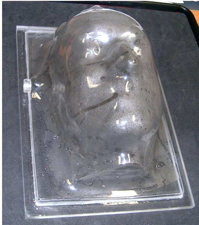
Figure 43: This miniature water tank was made for use with CT scanners. A plastic back panel was glued to the rectangular margin of a mask. It allows the same combination of uniquely shaped plastic mask and homogenous water fill, used in the linac experiments, to be imaged with CT.
