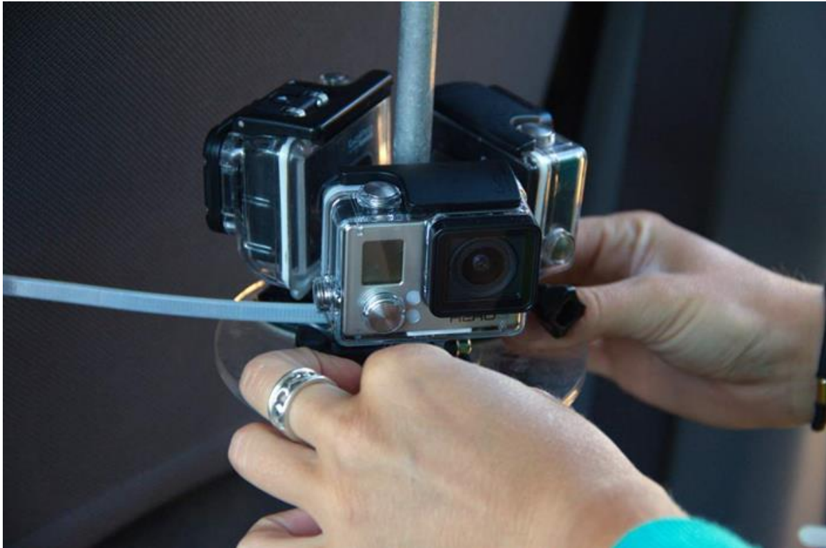
Figure 3. The GoPro mount on the novel stand method, for 360 degree video footage.
