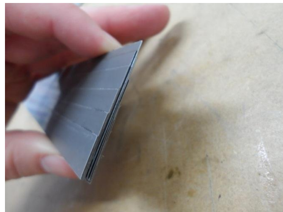
Figure 5 Left: Assembly process. Right: An assembled wedge of 10 laminations.
