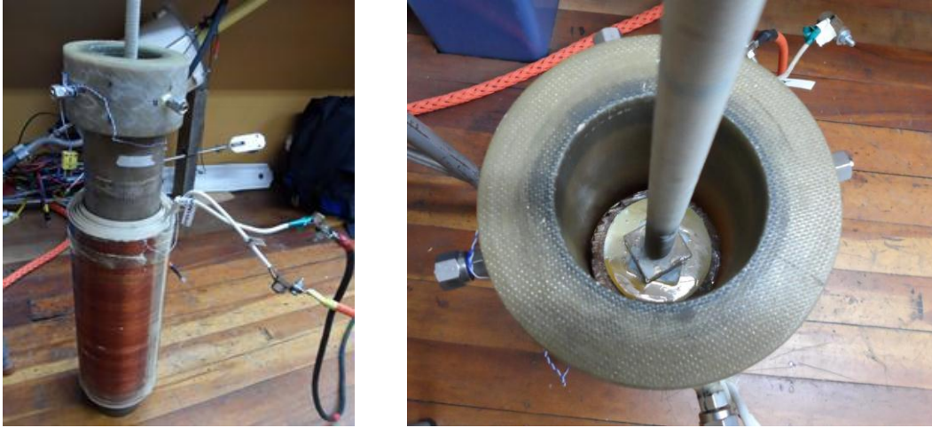
FIGURE 8: LEFT: COPPER WINDING TRANSFORMER. RIGHT: PARALLEL CORE SHOWN INSIDE PCT
