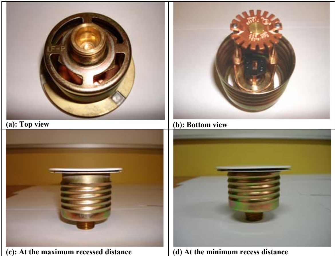
Figure 12.3: Sprinkler O_C at the maximum and minimum recess distance
