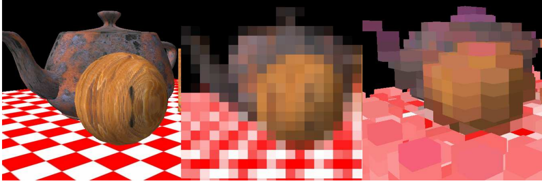
Figure 2.1: (a) An image, (b) pixels of an image at 34 \times 21 , (c) a rough voxel model at 20 \times 20 \times 20 .
