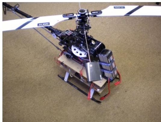
Fig. 2 Modified Trex600 with instrumentation equipment installed
