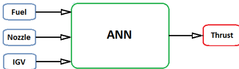
Figure 2.7: Block diagram of an ANN-based aero gas turbine model for system optimization consists of minimizing fuel while maintaining thrust [152].
