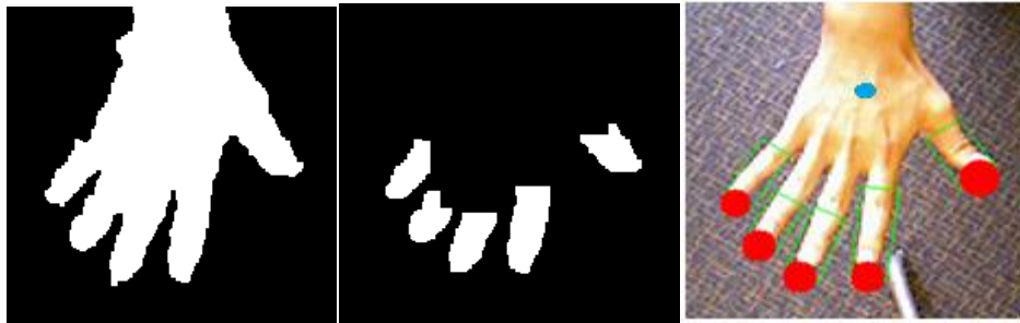
Figure 3.3: Filtrated hand region (left); Finger region (middle); Fingertips located (the blue point is the one has the maximum distance value in distance transformation) (right)
