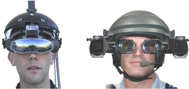
Figure 2.2: Video See-through HMD (left) and Optical See-through HMD (right)
