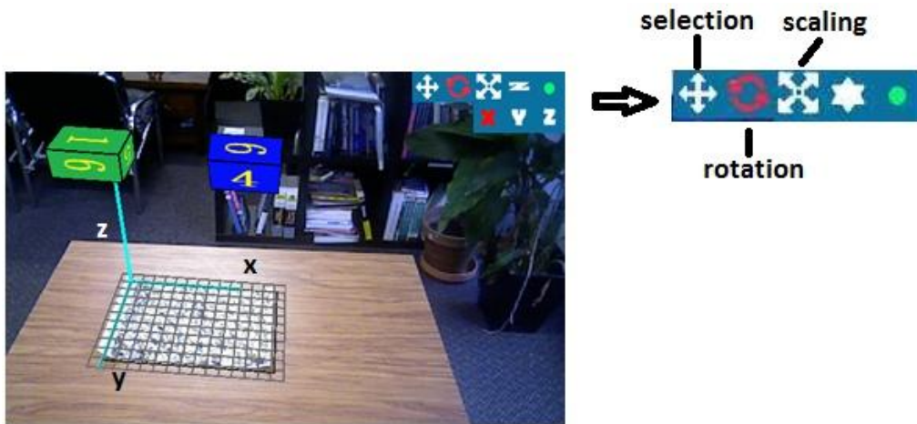
Figure 3.9: The mode menu and axis button are located on the top right corner, and activated ones are highlighted in red.
