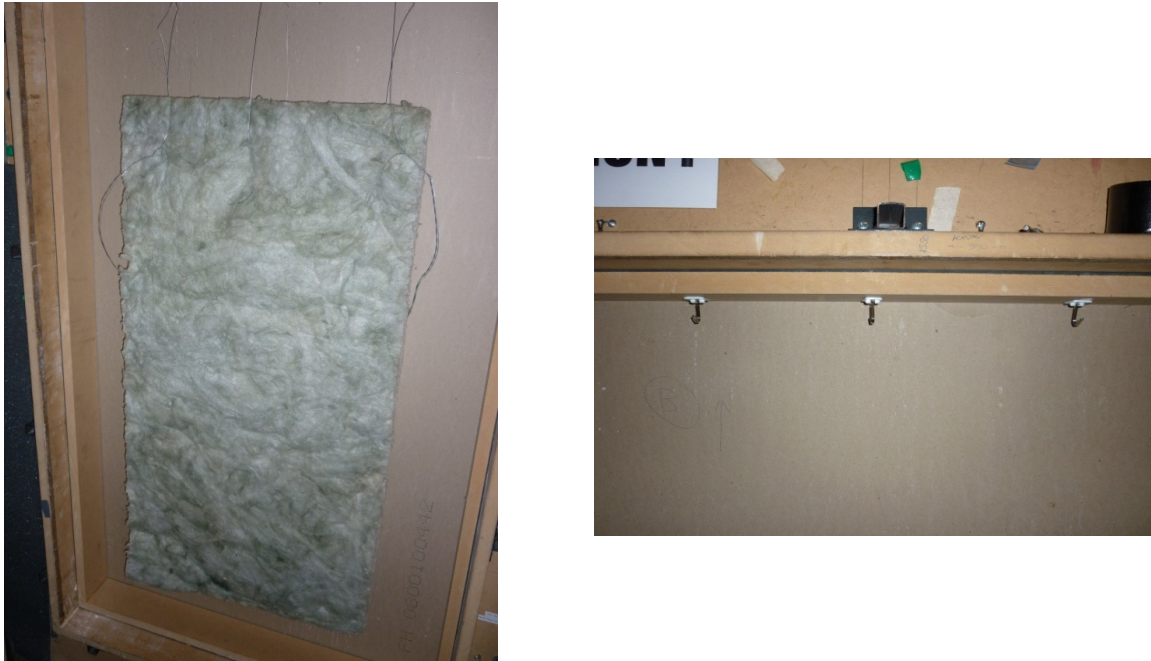
Figure 6 Mechanism used to suspend the glass-fibre within the 106mm deep cavity
