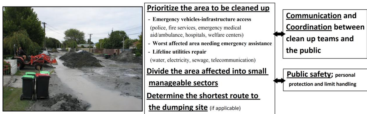
Figure 3: General strategy for Christchurch liquefaction clean-up. Photo: piles of liquefaction ejecta cleaned from residential properties and roads, ready for removal by heavy earth moving machinery at Bracken Street in the suburb of Avonside following the 22 Feb 2011 earthquake (Photo credit: Jarg Pettinga)
