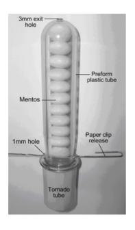
Figure 1. The delivery apparatus for the Mentos and Diet Coke activity. The total height of the apparatus is 18cm.
