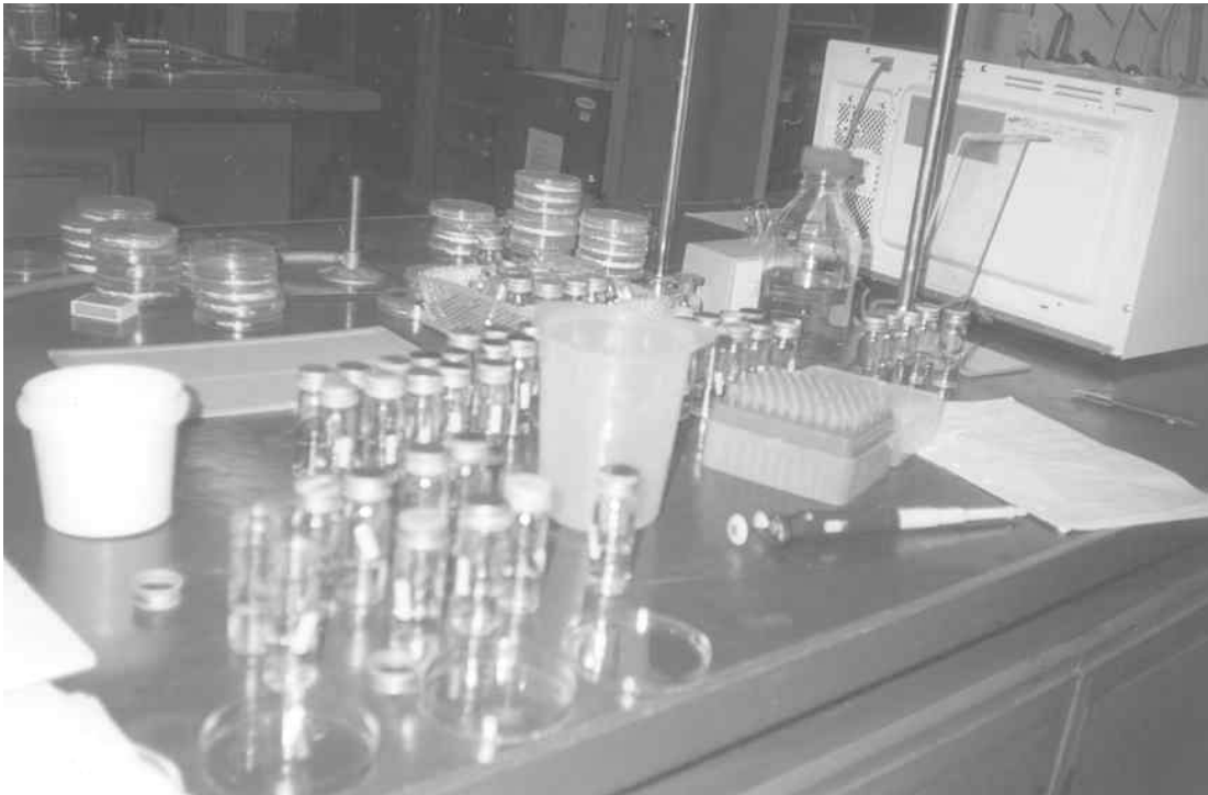
Fig 13. Preparing the SPC plates
