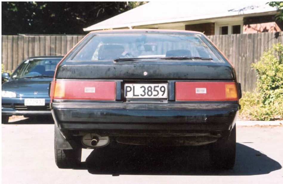
Plate Z.1 Elevational photograph of test vehicle for frontal area determination
