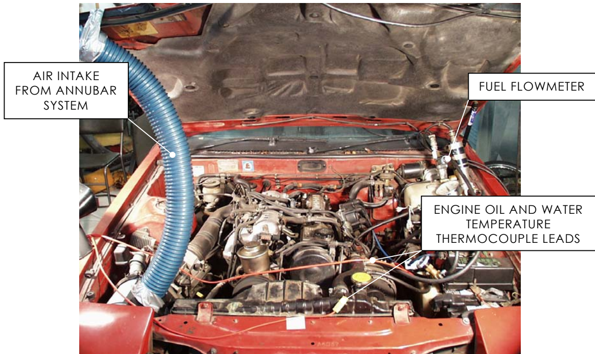
Plate 8.2 Test vehicle engine instrumentation
