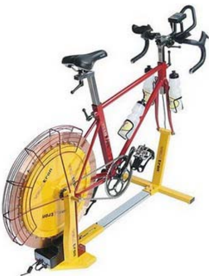
Figure 6. Velotron Cycle Ergometer used for the VO 2 max and MAP tests to determine aerobic capacity.
