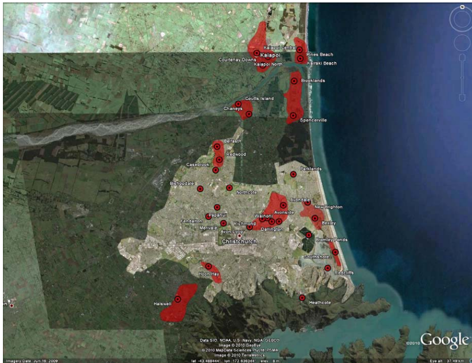
Figure 7. Areas of liquefaction (red shaded regions and red points) in Christchurch and Kaiapoi caused by the 2010 Darfield Earthquake (Cubrinovski et al, 2010).
