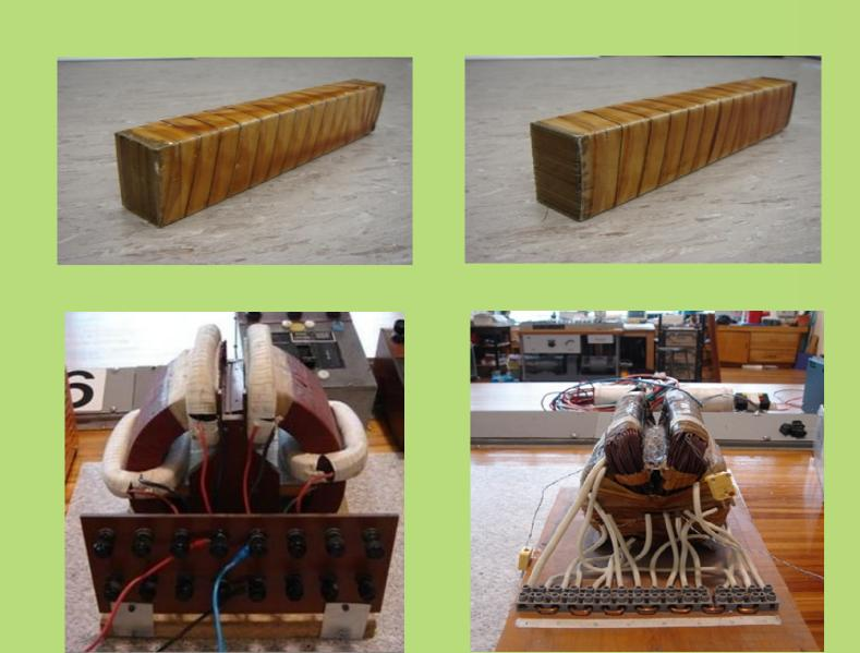
The arrangement included two billets with different orientated laminations, and two C-core uniform flux generator.
