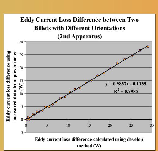
From the regression analysis results of two apparatus, the high correlations between calculated and measured values are turned. From the slope and the *R* vaule returned from regression analysis, the eddy current power loss in laminations from different directions can be accurately predicted using the new method.
