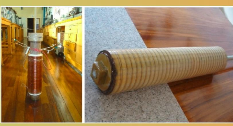
full core model, but retaining the core material inside the windings. This has been named the partial core transformer.
