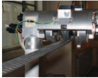
Fig. 22. Special running-gripping mechanism proposed in (Zhu et al., 2006)
