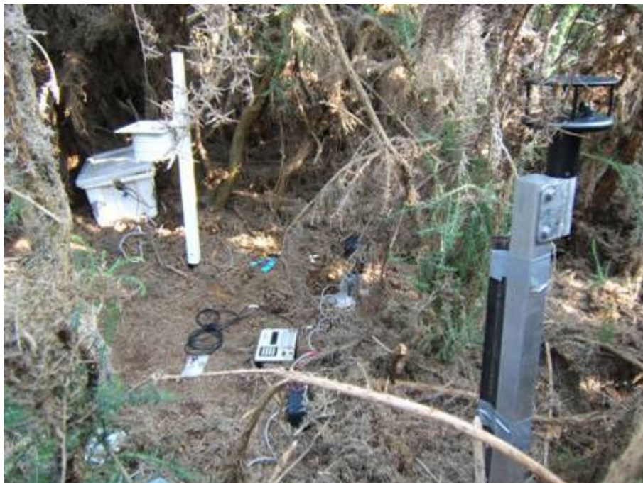
Figure 4.2. Instrumentation under the gorse canopy during hourly fuel moisture sampling on 12 December 2006. The photograph shows the temperature and relative humidity sensors (rear), pyranometer with datalogger (centre), and sonic anemometer mounted at 1 m above the ground (right foreground). The sonic anemometer at ground level is just visible, off centre to the right of the datalogger.
