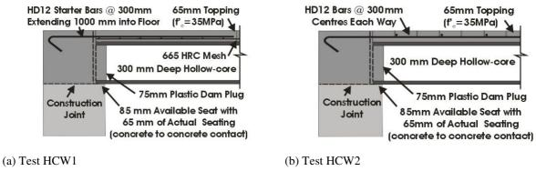
Figure 4 Connection details used in the two experimental tests
