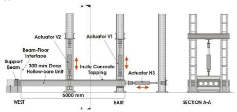
Figure 3 Single hollow-core unit and seating beam sub-assembly test rig used to subject the test unit to different load combinations
