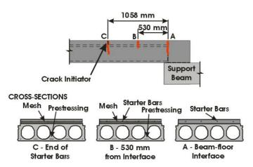
(a) Locations cracks formed in test specimen HCW1 during testing and cross-sections of the specimen at these locations
