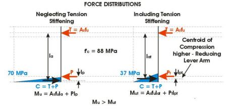
(b) Strains and forces in a prestressed hollow-core floor with topping containing mesh reinforcement
