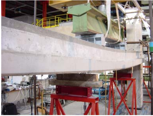
Fig. 9 – Global deflection of the Brooklyn suspended system
