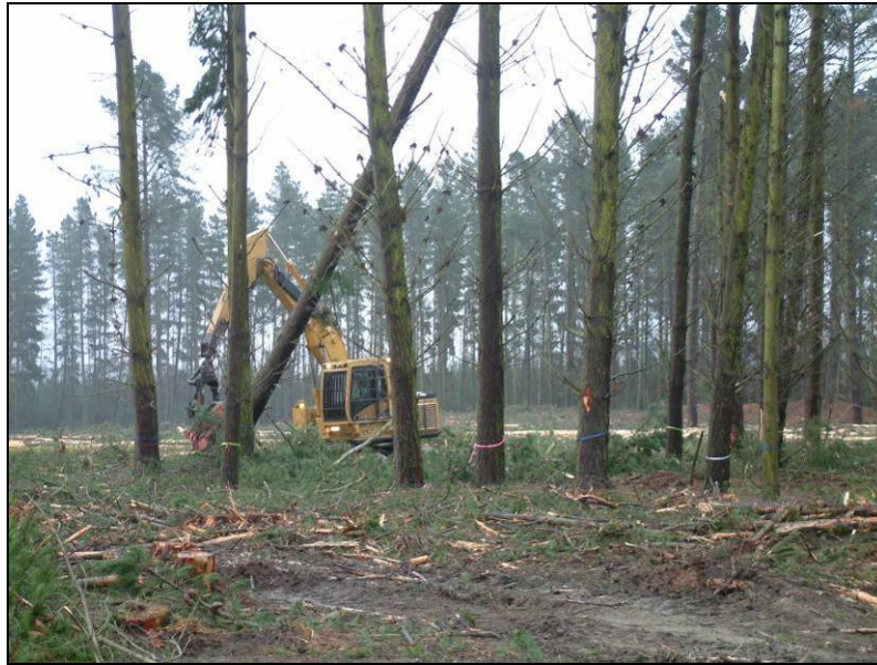
Figure 3: Waratah 622 with pine clearfell in Bottlelake Forest. Note that all trees are marked with unique colour-bands prior to felling.
