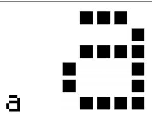
▲ A letter "a" from a computer screen and a magnified view showing the pixels that make up the image
