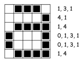
The picture above shows us how a picture can be represented by numbers. The first line consists of one white pixel, then three black, then one white. Thus the first line is represented as 1, 3, 1.
