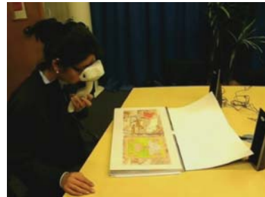
Figure 3: A user interacting with the book: tabletop setup with augmented book in the center, visualization through an AR handheld display, and background and 3d sound through speakers.
