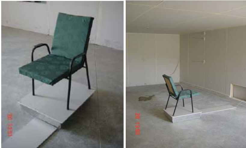
Figure 3. Upholstered chair in centre fire position (extracted from Bittern [10])
