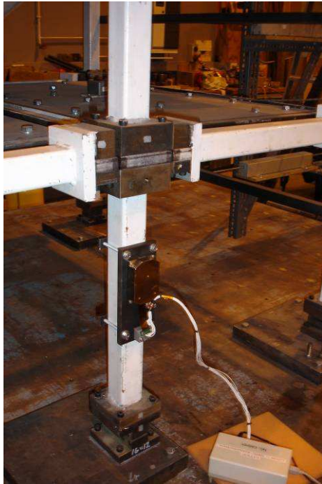
Figure 11. FOG attached to column.
