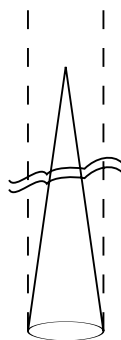
Figure 4.3 The limited height of laser guide stars compared to distant stars restricts its measurement of atmospheric turbulence.
