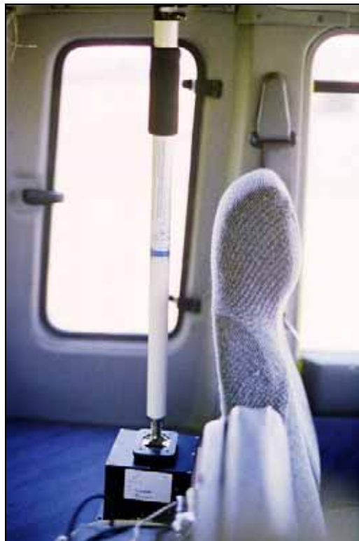
Figure 4.2 Gyro/accelerometer mounted inside test vehicle.
