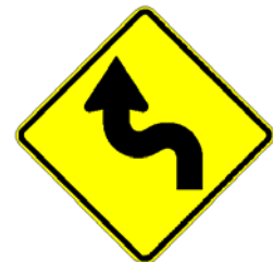
PW-21 Reverse curve of greater than 60° deflection
