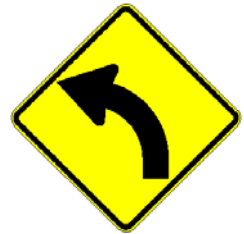
PW-17 Curve of less than 90° deflection
